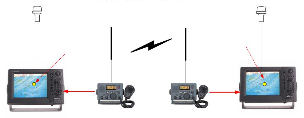
When any NavNet VX2 display is connected to the FM-3000 VHF radio, DSC position reports can be received from another DSC capable VHF transceiver, then shown on VX2's plotter as a waypoint. This capability allows two or more vessels to transmit their position to each other via VHF, then record that position information as a waypoint on the VX2's plotter.
